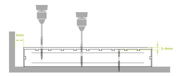
Keep the board 5mm away from the walls or other obstacles to allow for expansion of the composite products and also for ensuring good drainage and ventilation.
